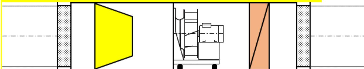
Air handling unit with in- and outlet pressure losses
